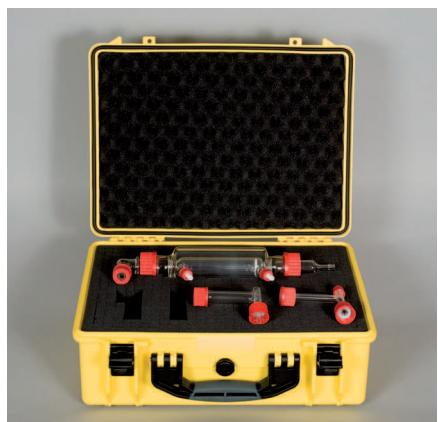
PCDD / PCDF sampling system with glass probe.
